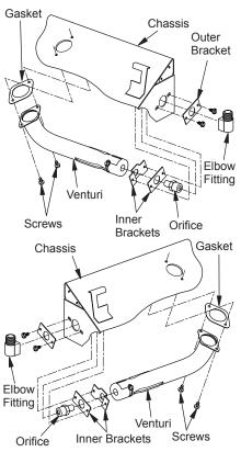
Figure 8 - Repositioning Gas Inlet to Left Side of Unit
